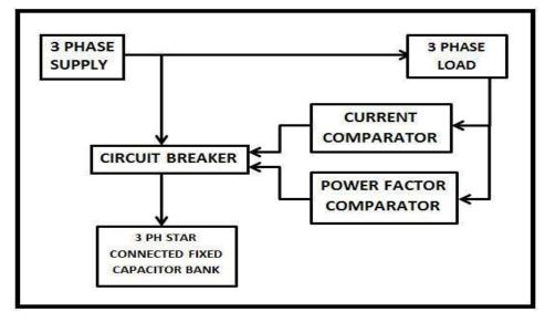
Figure 4: Block Diagram of Compensated System with Fixed Capacitors
