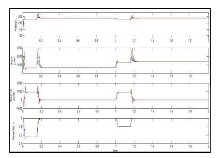
Figure 5: From Top to Bottom- Voltage, Active Power, Reactive Power, Power Factor of Phase a
