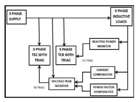
Figure 6: Block Diagram of SVC with Feedback
