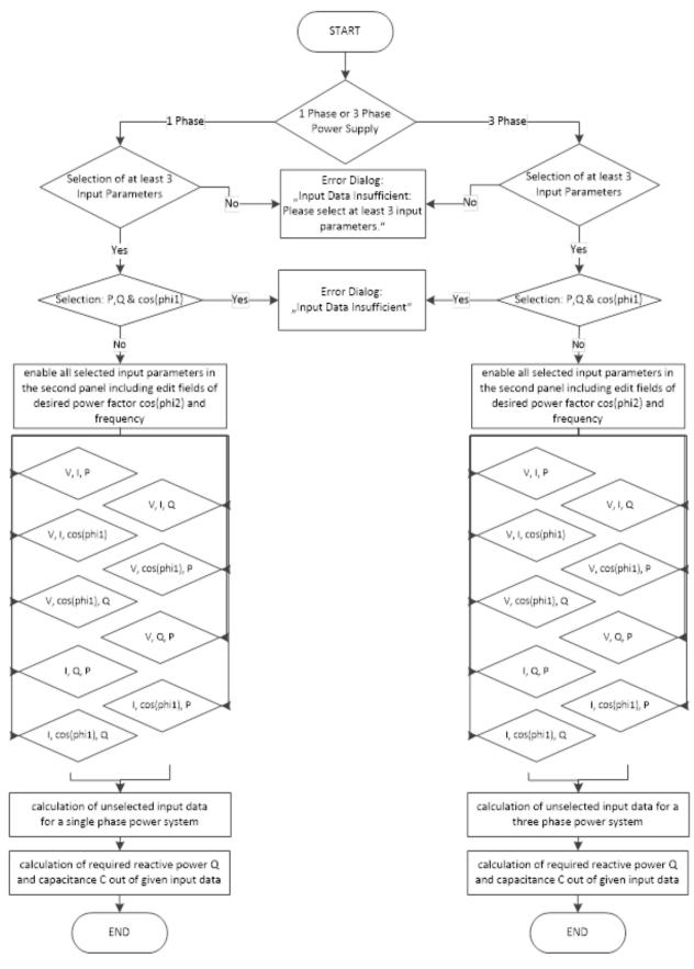
Figure 1: Flowchart Representing the Calculations Done in GUI
