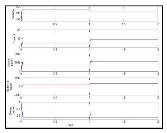
Figure 3: From Top to Bottom - Voltage, Load Current, Active Power, Reactive Power, Power Factor of Phase a
